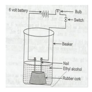
Material required: - Beaker, nails, battery, connecting wires, bulb, switch and alcohols.
